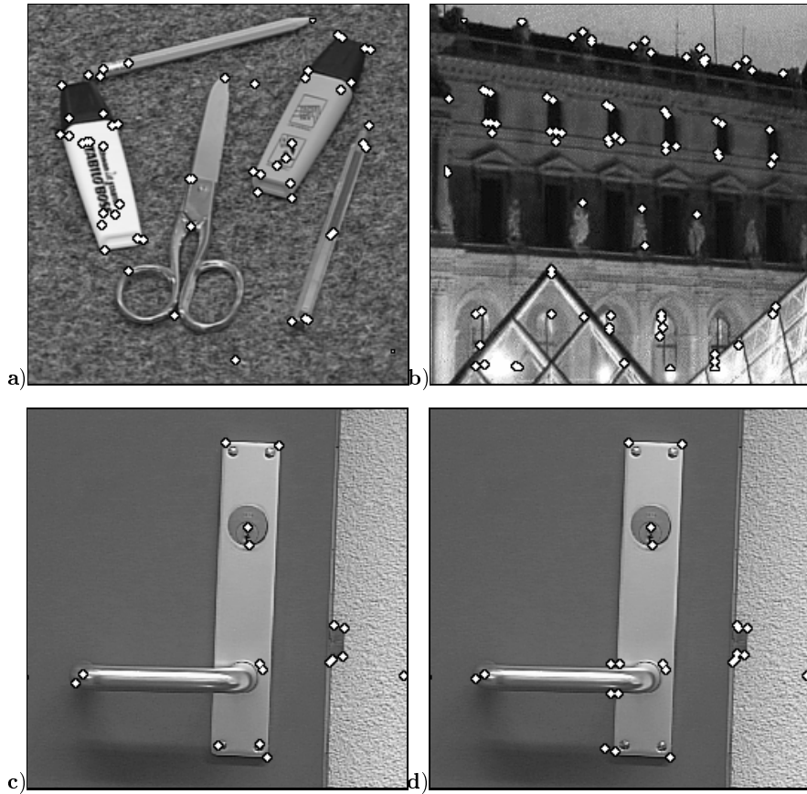
Fig. 2. Detected corners in a variety of natural images. a) to c) show corners found in the grey-level image, d) the ones in the color image corresponding to c) . The parameter values for these results have been N = 8 , \sigma_{min} = 1.18 , \sigma_{max} = 9.43 , S = 15 .
